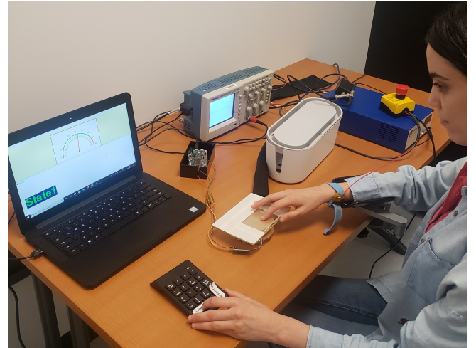
Fig. 7: Experimental setup including electrovibrating surface, load cell, signal generator, keypad and computer monitor.
