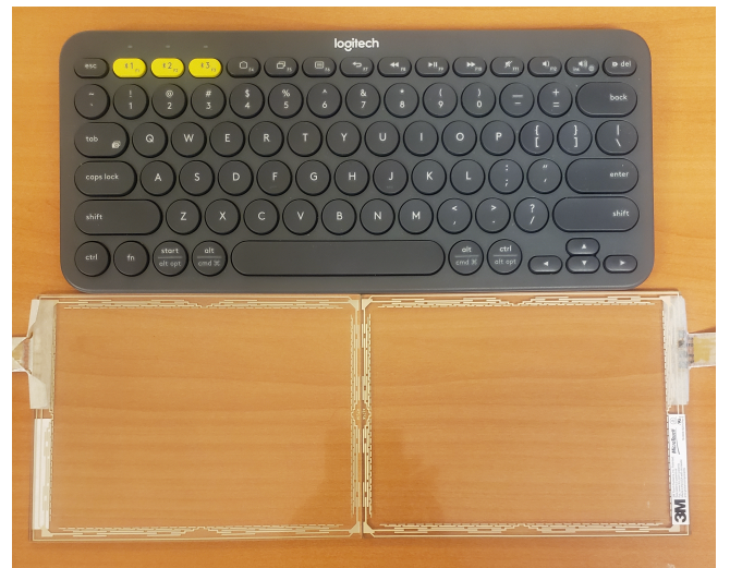
Fig. 5: Sketch of electrovibrating keyboard made with an off-the-shelf keyboard and two capacitive plates.
