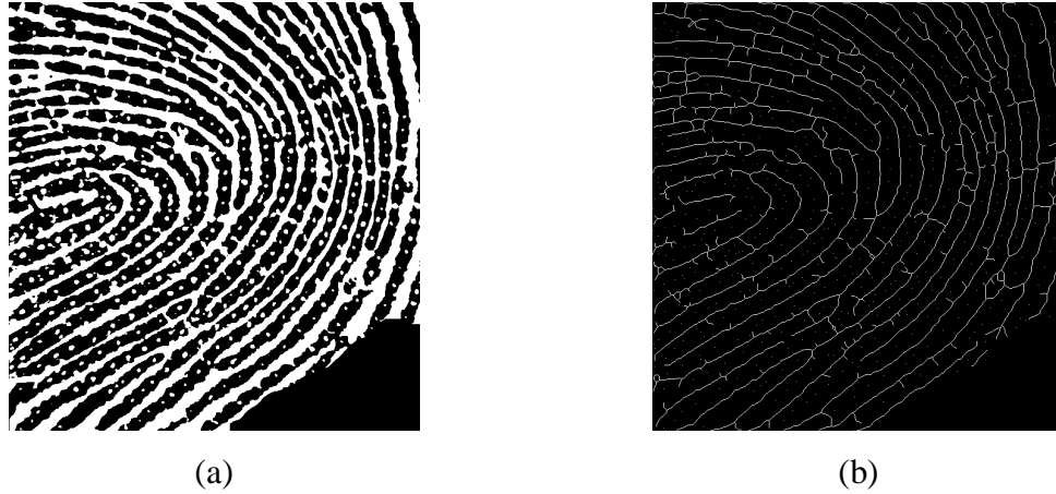
Figure 28. Thinning example: (a) binary image, and (b) thinned image.
