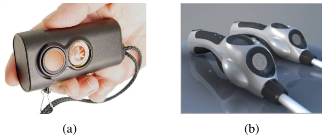
Fig. 2.1 Examples of electronic mobility aids: (a) the MiniGuide and (b) the UltraCane. (Pictures used with permission from GDP Research and Brian Hoyle respectively.)
